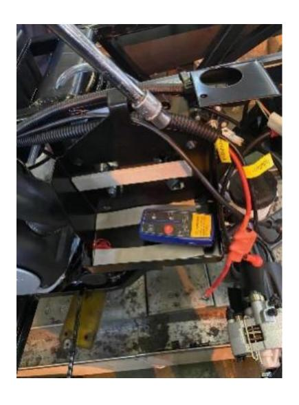
步骤六:将绞盘开关安装到左侧龙头把手上(走线需要将前面塑料盖板拆除) 6. Install the winch switch to the left side of the handle bar by removing the handle bar cover. (See pic)
