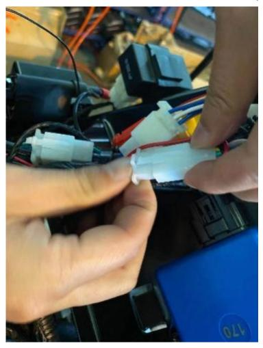
步骤八:将绞盘开关上的红线,与车子主电缆上的端子对插(每台车上都有此端子) 8. Connect the red wire of the winch switch to the terminal of ATV wire harness. (See pic).
